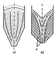
By definition, these are the only flow profiles, i.e. mass flow in which the whole bulk material starts moving when discharging the silo, and funnel flow in which dormant zones exist.
