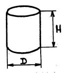
Drums are usually cylindrical or roughly cylindrical and are defined by their height (H) and (maximum) diameter (D).
